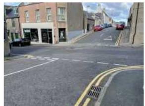
*“Tactile paving is missing at all junctions along Duff Street.”*
